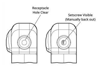
NOTE: Contrast between a clear and a blocked receptacle hole. Applies to single or dual pin headers.
