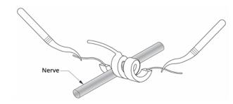
5. Pass the *distal* suture portion of the helical under the nerve and back around so that it encircles the nerve.
