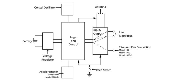
For descriptive purposes, the generator circuitry is divided into functional sections as shown in the table below.
