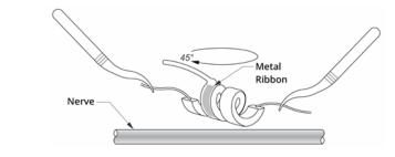
4. Place the turn of the helical where the lead wire connects to the helical (the section with the metal ribbon) onto the nerve.
